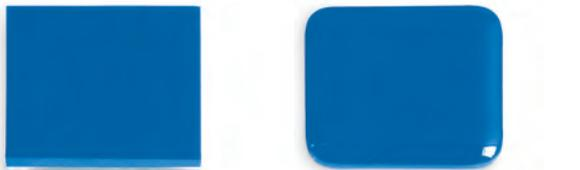
Figure 1: Two, 1/8" (3 mm) layers fired to 1500°F (816°C).
