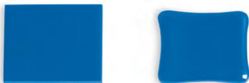
Figure 3: One, 1/8" (3 mm) layer fired to 1500°F (816°C).
