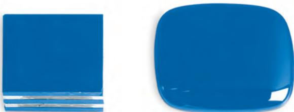
Figure 2: Five, 1/8" (3 mm) layers fired to 1500°F (816°C).
